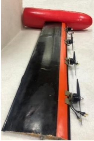
Figure 4. The electric motor was located on the leading edge of the wing
