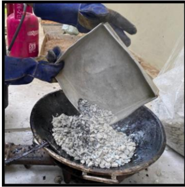
Figure 2.a Porous Asphalt Mixing Process
