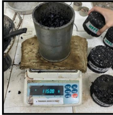
Figure 2.b Test Specimen Molding Process
