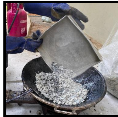
(b) The aggregate was added into the mixture of asphalt and HDPE plastic.
