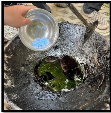
(a) HDPE plastic was first added to the asphalt
