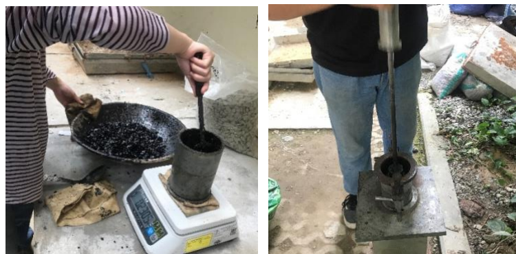
Figure 4. Printing and compaction of test specimens
