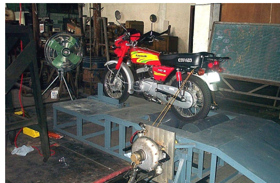
Figure 15. The Chassis Dynamometer and the Mounted Test Motorcycle
