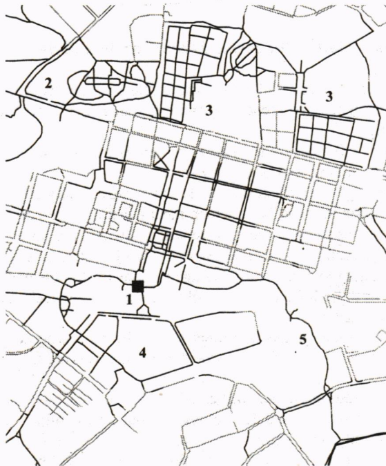
Figure 6. The secure (light grey) and insecure (black) pedestrian network around the railway station in Alingsås . Scale 1:13 000.
