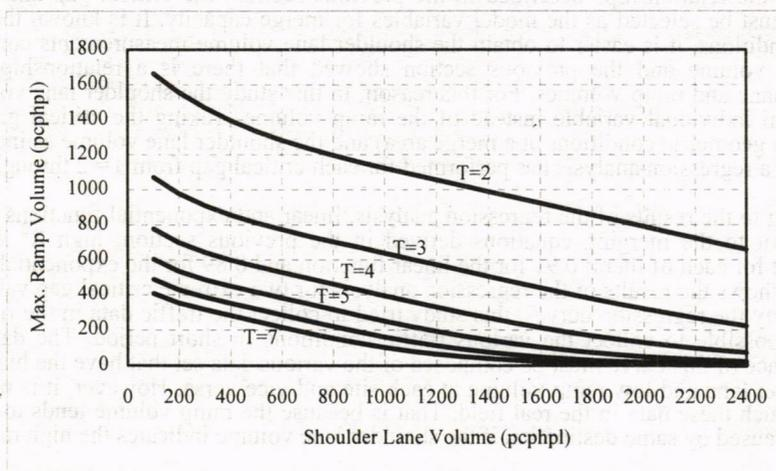
Figure 3. The Ramp Capacity under Shoulder Lane Volume ( $K=2$ )
