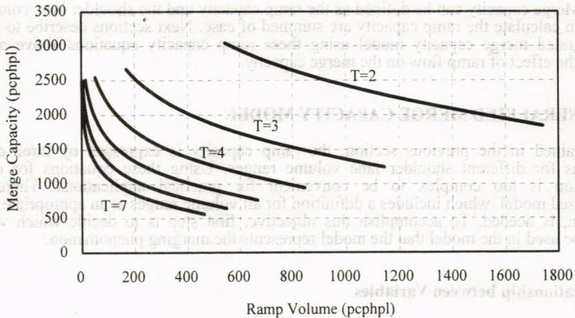
Figure 4. Relationships between Ramp Volume and Merge Capacity ( $K=2$ )
