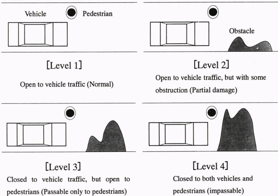
Figure 5. Extent of Road Blockage in Four Levels
