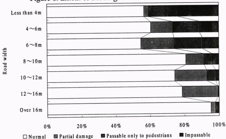
Figure 7. Ratios of Blockage Levels by Road Width (in total road lengths)
