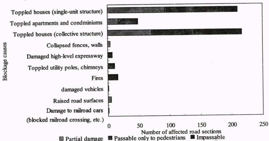
Figure 8. Frequency of Main Road Blockage Causes by Road Section
