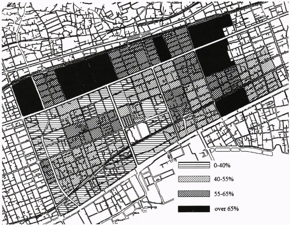
Figure 4. Structure Collapse Ratios in Town Blocks
