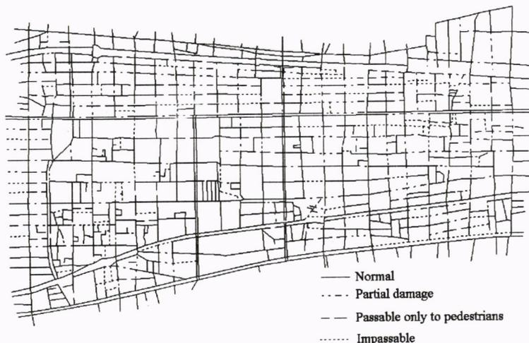
Figure 6. Extent of Blockage on the Road Network
