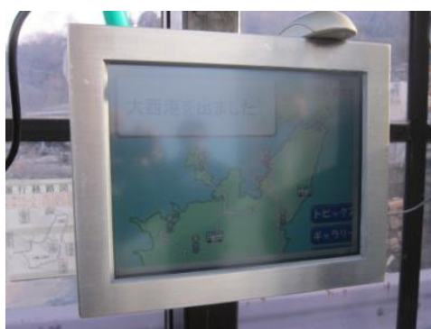
Figure 2. A touch panel terminals installed at the bus stop
