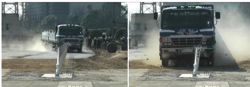
Figure 19. Post-collision swept path of the large vehicle
