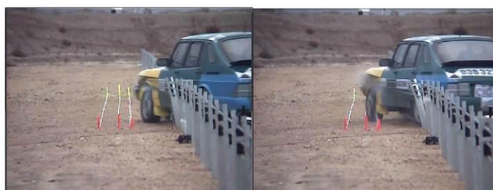
Figure 5. Crash test involving a wire rope guardrail system (from the CASS Cable Safety System Product Manual)
