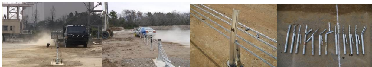
Figure 11. Conditions of the new wire rope guardrail system upon collision and thereafter
