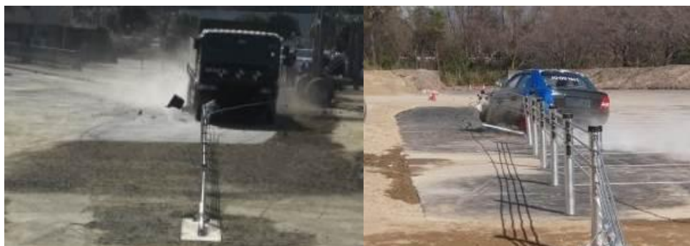
Figure 13. Collision with the improved wire rope guardrail system
