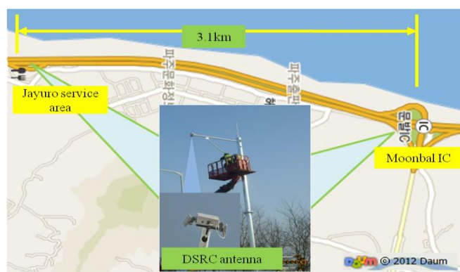
Figure 3. Data collection area and DSRC antenna
