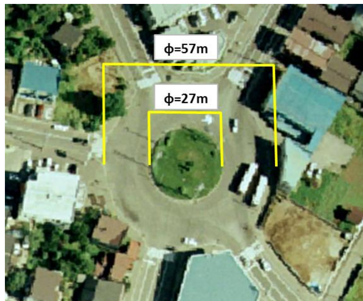
Photo 3. Rotary intersection (Sakura, Otaru)
