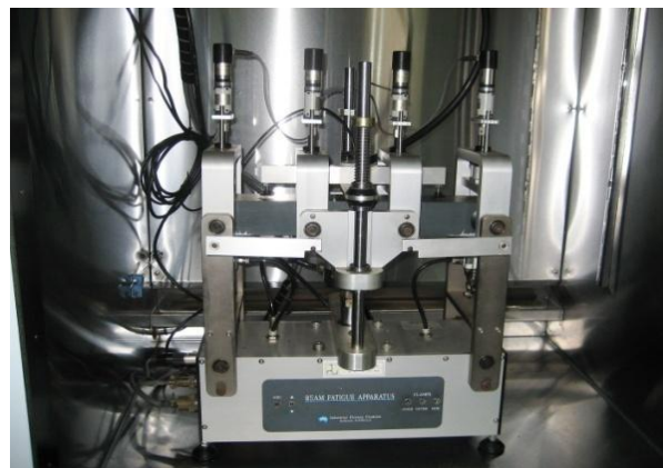
Figure 5. Four point bending test apparatus
