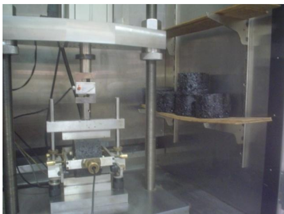
Figure 4. Indirect tensile test apparatus
