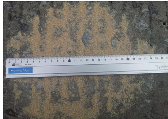
(a) Sand Patch Test on the Asphalt pavement Section (B) Sand Patch Test on the Concrete Pavement Section
