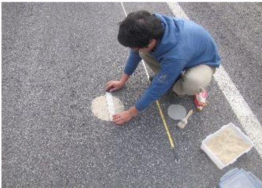
(a) Sand Patch Test on the Asphalt pavement Section (B) Sand Patch Test on the Concrete Pavement Section
