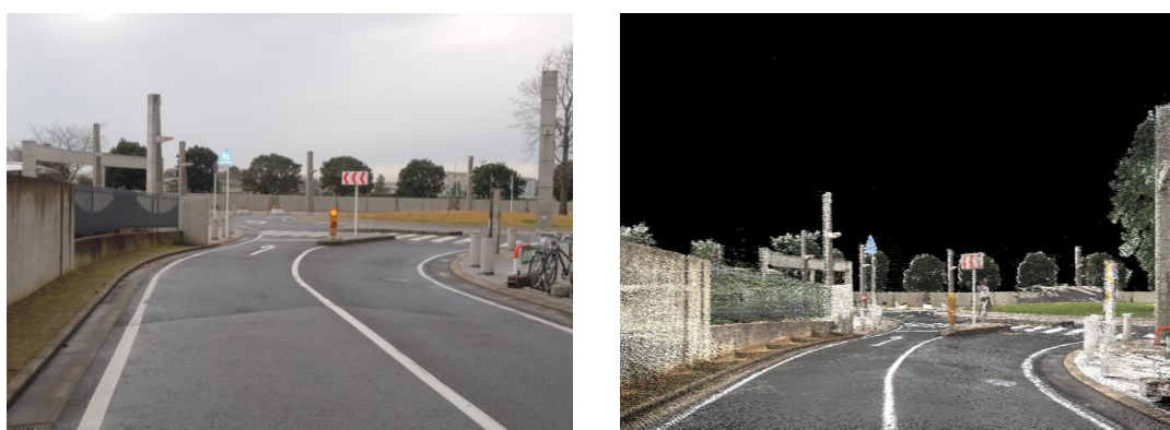
Figure 2. Example of road section (left: photograph, right: point cloud data)
