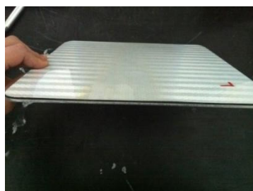
Figure 4. Concept of road sign with insulation inserted which was used in the experiment
