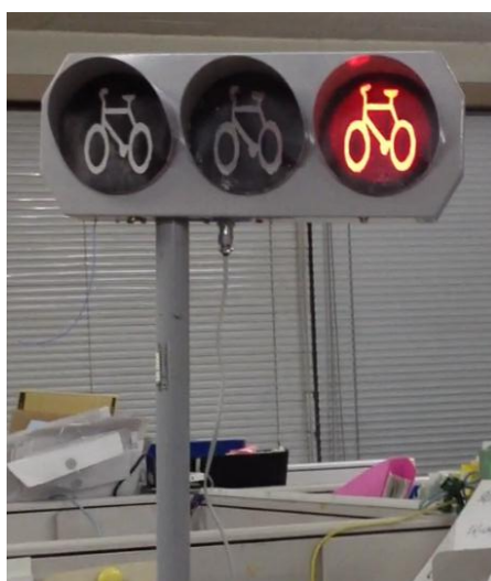
Figure 7. “Bicycle signal” modified from small scale traffic signal
