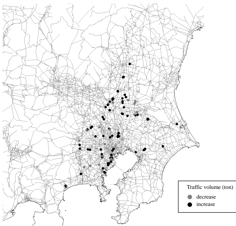
*Intersections with turning hindrance that had changes by traffic assignment are shown. Figure 15. Intersections with changes in traffic by traffic assignment (Case 3 – Case 1)
