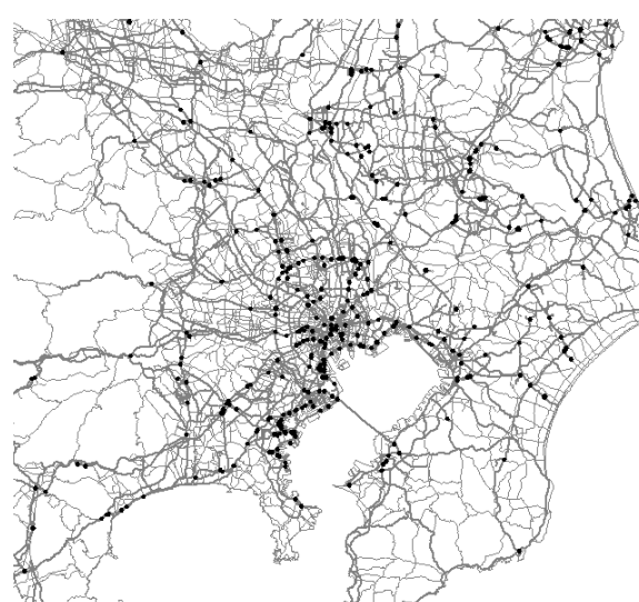
Figure 9. Intersections on Weight-Designated Roads where 40 ft containers are not able to turn
