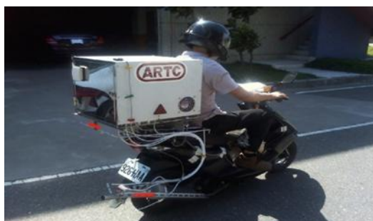
Figure 2. OBS-584 installed onto the test scooter
