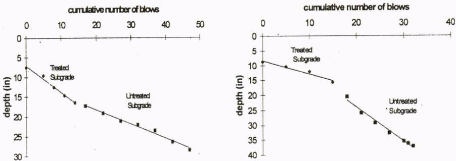
Figure 7. DCP Data from IH30 for Treated and Untreated Layers
