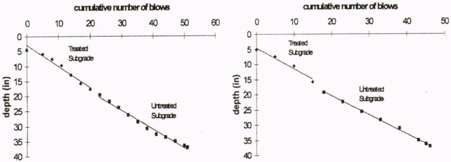
Figure 6. DCP Results from FM2818 for Treated and Untreated Layers
