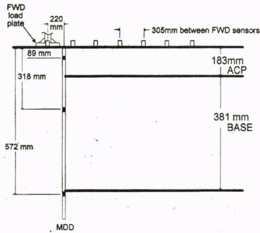
Figure 3. Schematic of FWD-MDD Test
