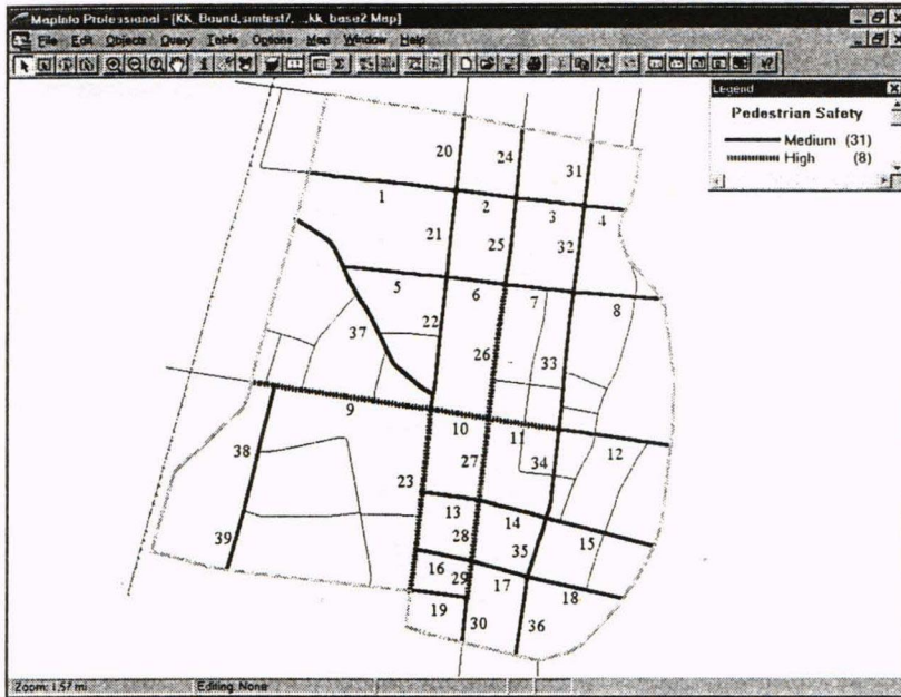
Figure 9. The ES indices of all links in the Khon Kaen road network for pedestrian safety
