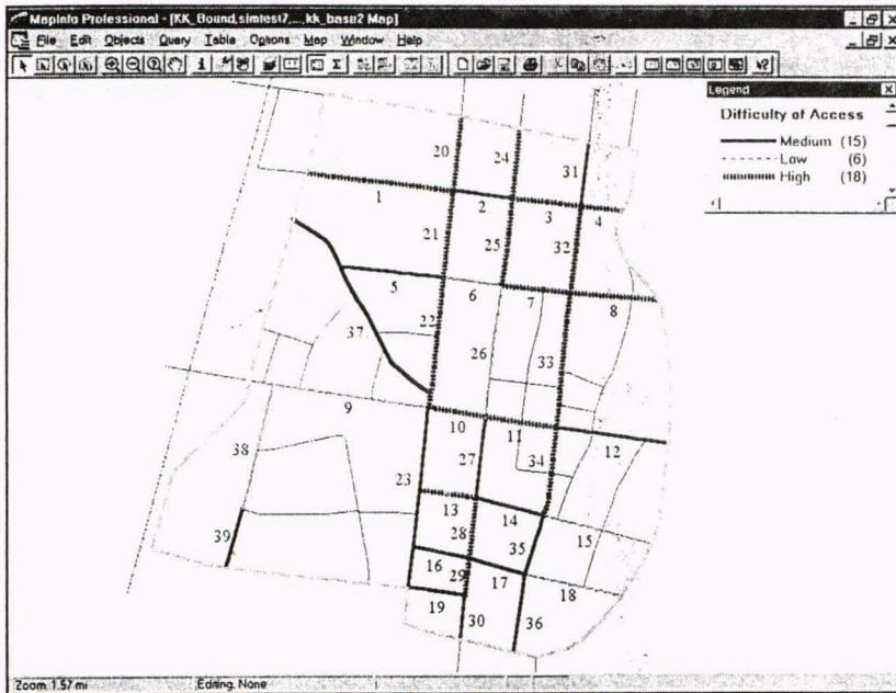
Figure 7. The ES indices of all links in the Khon Kaen road network for difficulty of access
