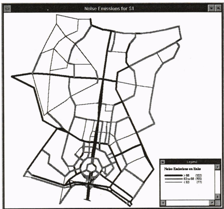
Figure 2: Noise emissions from each link at a facade 10 m from road centre line. No facade correction is applied. (Number of links in each class intervals are given in brackets)
