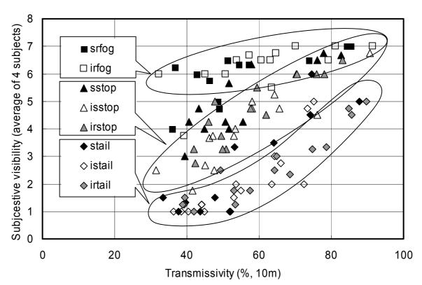
Figure 5 Subjective visibility assessment value versus transmissivity at 10 m as a function of the eight rear lamps.
