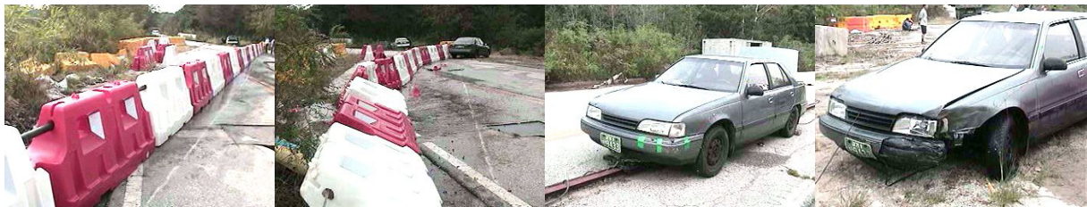
Figure 4. The testing vehicle and barrier before and after the collision test - Guard Box
