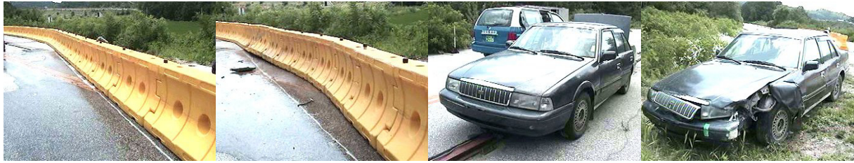
Figure 3. The testing vehicle and barrier before and after the collision test - Green Safety Box
