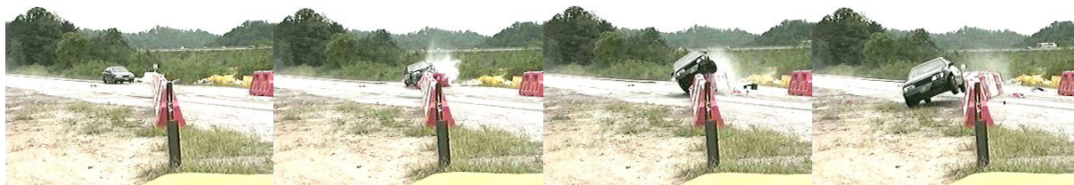
Figure 2. Real Collision Testing Against Guard Box
