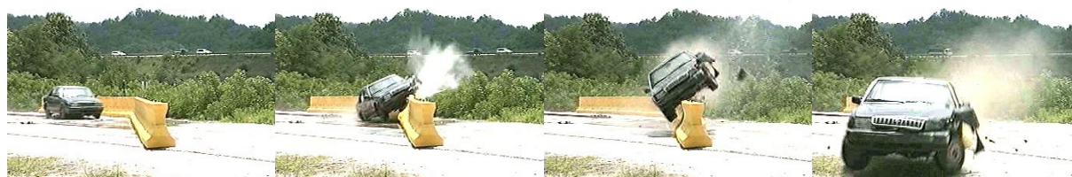
Figure 1. Real Collision Testing Against Green Safety Box
