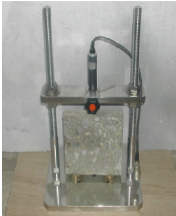
Figure 4. Picture for the AASHTO-type Device of the CTE Test
